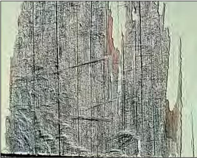
**Figure 17. Severely weathered wood surface.**
