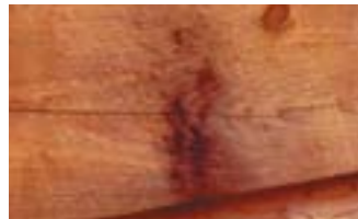
Dark colored streaks from metallic tannates. Oxcon solution will remove rust stains caused by nails, screws and fasteners.
