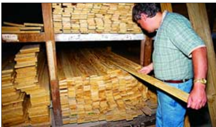
Once delivered from the mill to the dealer, Southern Pine flooring should be stored in a clean, dry, enclosed building.
