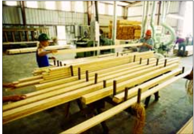
At the mill, flooring is sorted according to grade and length.
