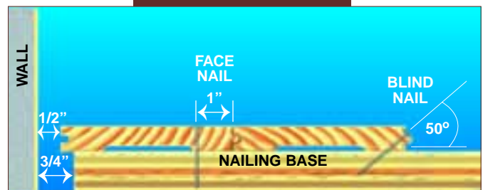
Figure 11: Nailing Detail
