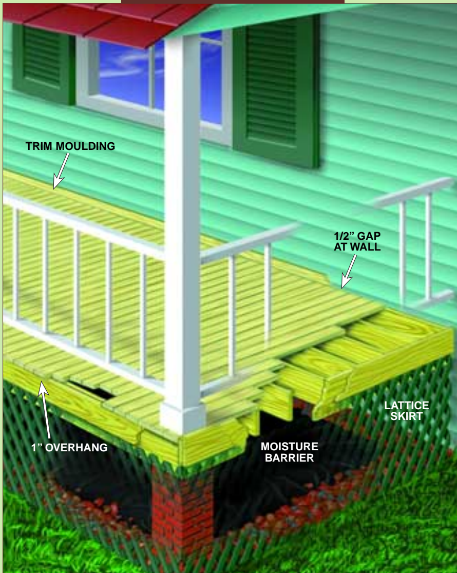
Figure 14: Porch Flooring Details
