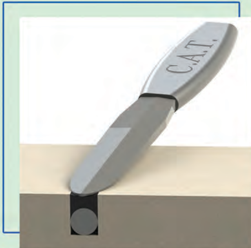
Caulk Application Tool invented by Wayne Belcher
